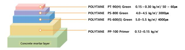
Paint requirements; surface conditions, work methods, depends on the working conditions.
